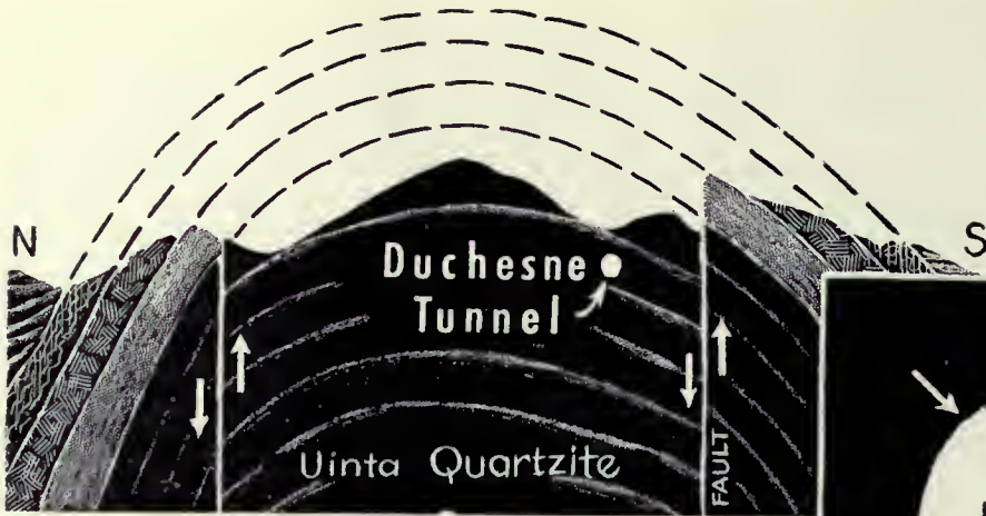
HOT ROCK folded in under great pressure millions of years ago, now hard and cold, is shown above in this artist's drawing of a section of Duchesne Tunnel.
